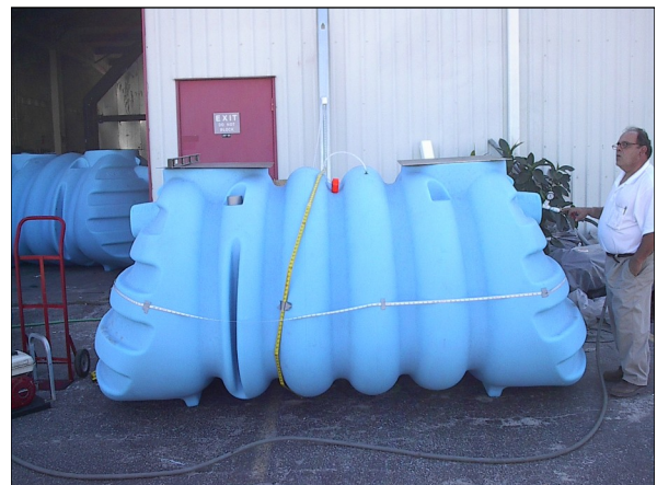
1,250 Gallon Tank Under Vacuum (44.50" of Water)
