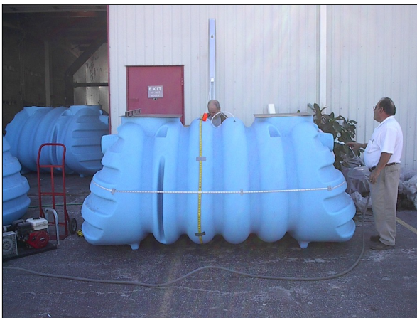
1,250 Gallon Tank Under Vacuum (33" of Water)
